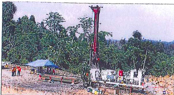
Dando Mintec 12.8 being used for coal exploration for a major customer in Indonesia
