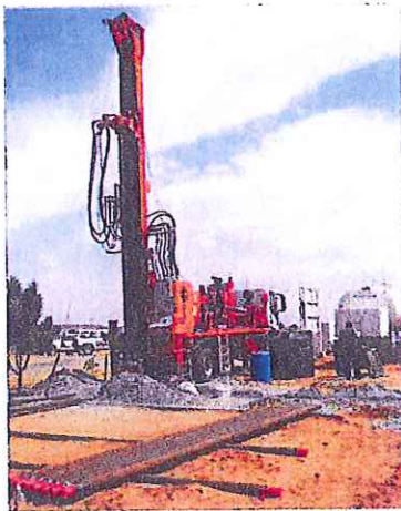
Near right: the Watertec 24 is capable of drilling down to 830m
