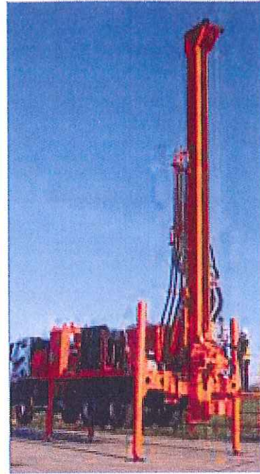
Far left: Dando supplied this bespoke Watertec 12.8 water-well drilling rig to the British Army
