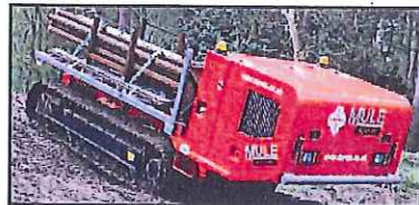
Dando has recently diversified into the tracked utility vehicle market with the launch of the Dando Mule ATV5-RC- a remote control self loading/unloading crawler carrier.
